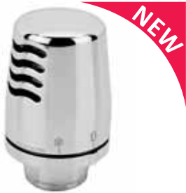
Art. 1099 Thermostatic head with liquid sensor for thermostatic valves for radiators. Temperature locking and limiting to a desired value with a forked pin system (see page 2). Chrome finish.
